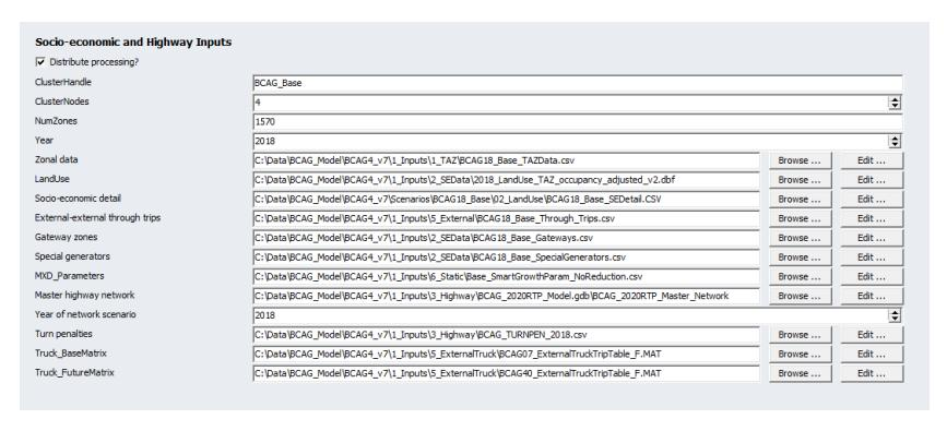
The Browse boxes are used to search for the input file and the Edit boxes are used to edit the file within Cube.
